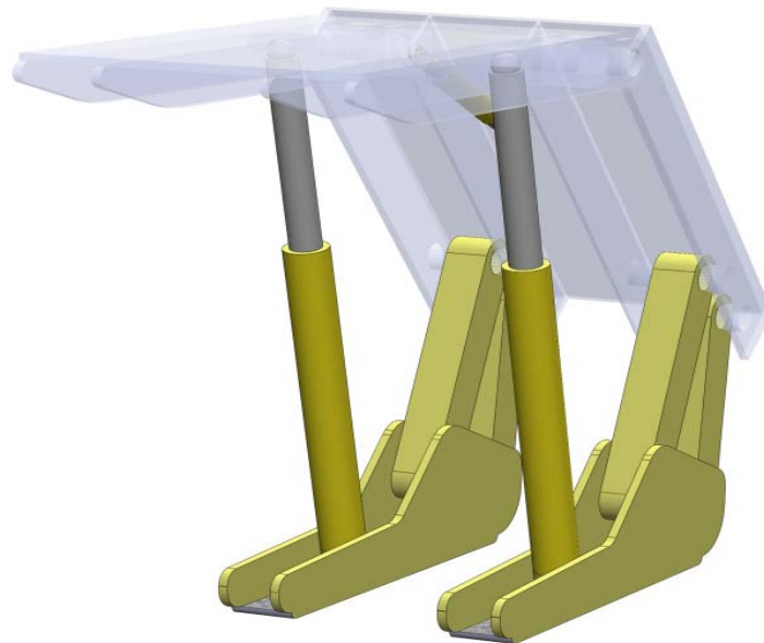
Fig.1. Model of the powered roof support
